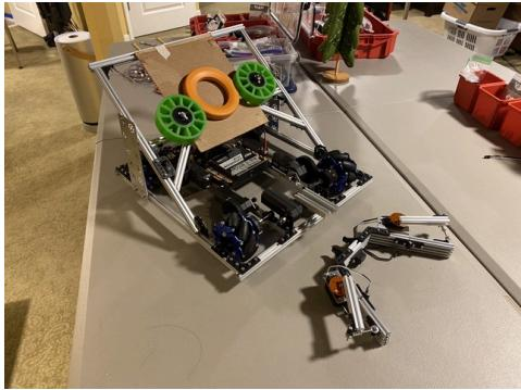
We had a few problems with the overall design. Since the robot had to fit in an 18 inch by 18 inch square, our back motors were pointed up at an angle because there wasn't enough space. So we adjusted the chassis and the fit, and the battery and hub fit snugly in the middle. But to accomplish this we had to flip some hex motors so we had to change some programming. At this point we have also attached the grabber and shooter to the robot. We also had to alter the design to fit a camera on.
