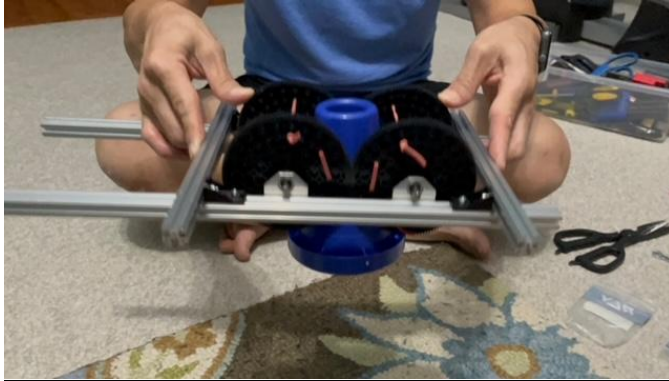
Figure Q: First prototype of rubber band grabber to see if it would be faster.
